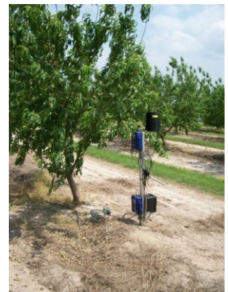
Figure 1 - Field Station automatically measuring and transmitting tensiometric soil moisture and other soil indices at various depths.
