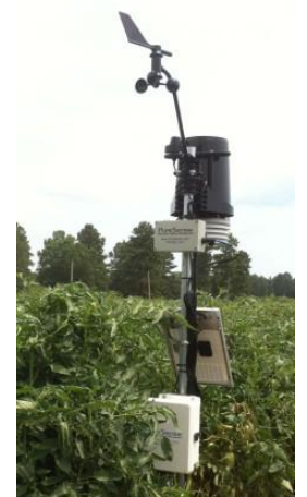
Figure 2 - Field Station continuously measuring and transmitting volumetric soil moisture and salinity (at various depths), weather (in and out of canopy), and irrigation system pressure (indicating when irrigation is occurring).
