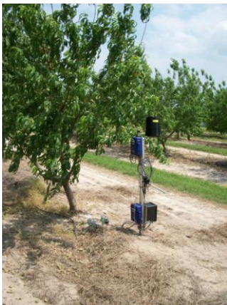
Field Station continuously measuring and transmitting tensiometric soil moisture and other soil indices at various depths.
