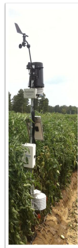
Field Station continuously measuring and transmitting volumetric soil moisture and salinity (at various depths), weather (in and out of canopy), and irrigation system pressure (indicating when irrigation is occurring).
